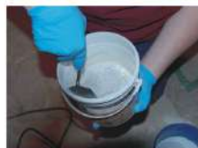
Mix resin & hardener together 9:1 ratio
